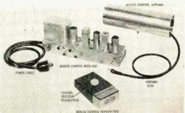
Fig. 9. A good portion of the receiver signal circuits is included in the remote-control box of the TechMaster unit.
