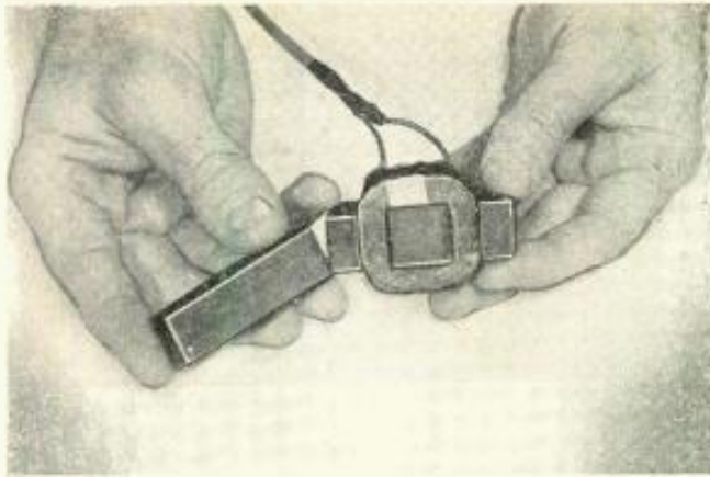
Fig. 4. In order to increase the pickup sensitivity of the choke it is necessary to take one side of the core off as shown. Most laminated cores will come apart quite easily.
