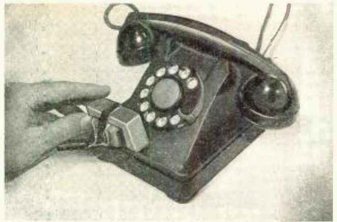
Fig. 5. In recent model telephones the pickup choke will work well in the area shown here or on the side. For telephones with metal housing the best spot is under the phone.
